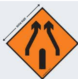
WK 017 - End of Obstruction Between Lanes
